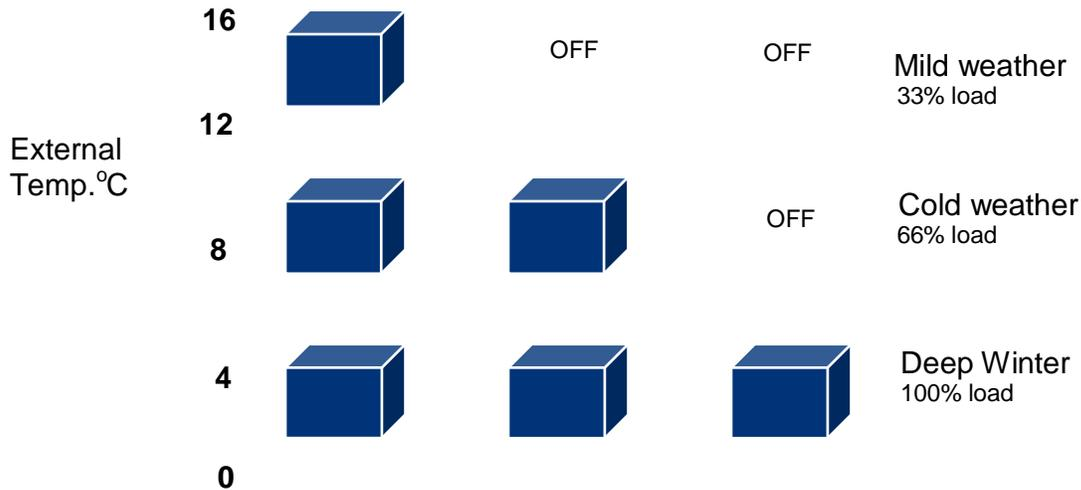
One boiler operating at full or near to full capacity will operate more efficiently than multiple boilers running at part load. The Site Manager should be tasked with ensuring only the minimum necessary number of boilers is switched on, depending on external air temperatures. This may require some experimentation. If you are still unsure, consult the County Councils Property Maintenance or your local heating contractor.
