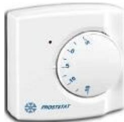
The frost stats are typically located in the boiler house and should be set at no higher than 3°C. As these thermostats operate independently of the system’s time control, they can be responsible for heating systems switching on unnecessarily if set too high. The effect of this can be most accurately verified from interrogation of AMR data. If you are unsure whether you have access to AMR data, check with the Energy Management Section.
